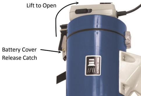
Insert 8 x C type batteries into the 2 carriers(4 in Each), observing the correct polarity, then return the carriers to the megaphone aligning the + ve and - ve terminals of the carrier with the terminals in the megaphone. Replace the cover and securely replace the catch and push closed.
